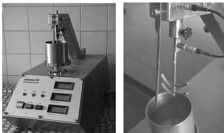
Fig. 1. Viskomat PC and its measuring element
